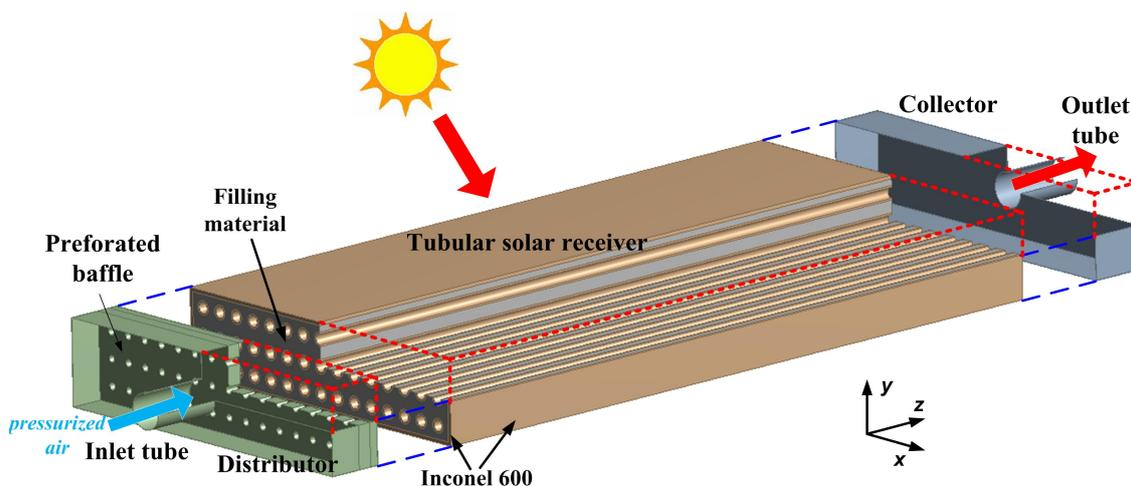
Fig. 1: Schematic view of the tubular solar receiver equipped with an inlet fluid distributor and an outlet fluid collector.
